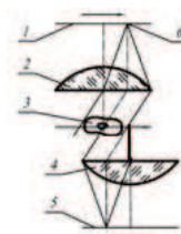
Fig. 2. Scheme sensing an object in microscopy with broken optical axis.
